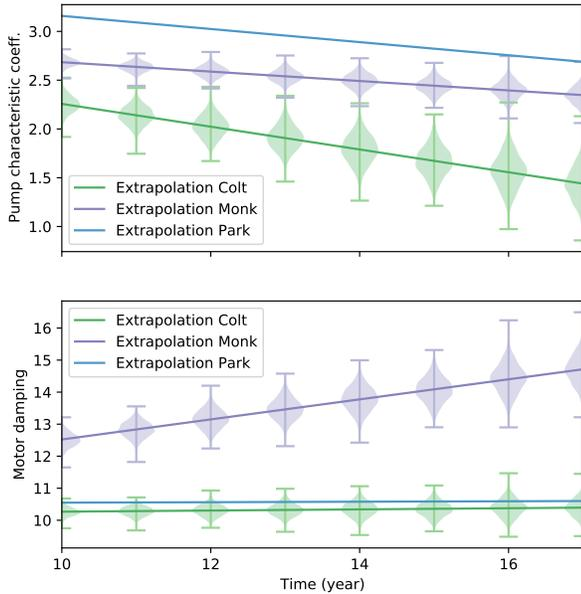
Fig. 8. Marginal probability distributions of degradation parameters for the units Colt and Monk.
