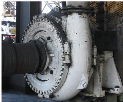
Fig. 1. Example of a centrifugal pump [3].
